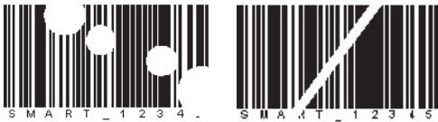
Reading of damaged codes thanks to SMART
